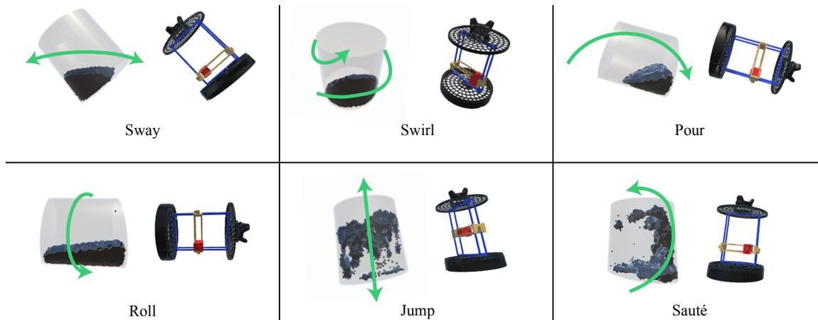
Figure 2. Six different actions for interacting with the SWISH haptic input system
