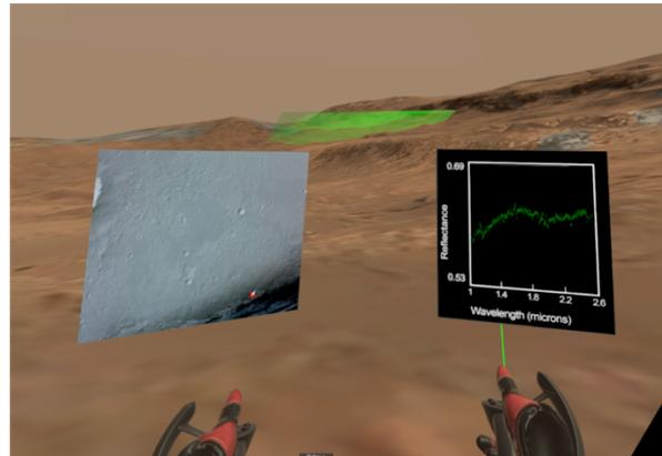
**Figure 1:** This VR environment provides the user with a first-person perspective on Curiosity rover images. The green polyhedron represents the intersection of an orbital CRISM pixel footprint with the 3D surface. The user's other displays include a local map of the rover's traverse for navigation, and a plot of CRISM spectroscopic data corresponding to that pixel.
