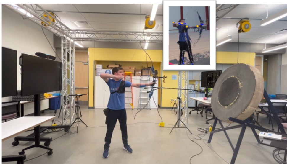
Figure 1: Augmented Coach demo setup, comprising Kinect cameras, Meta Quest headsets, and TV displays for observation. Inset: Volumetric annotated view of athlete in Meta Quest headset.
